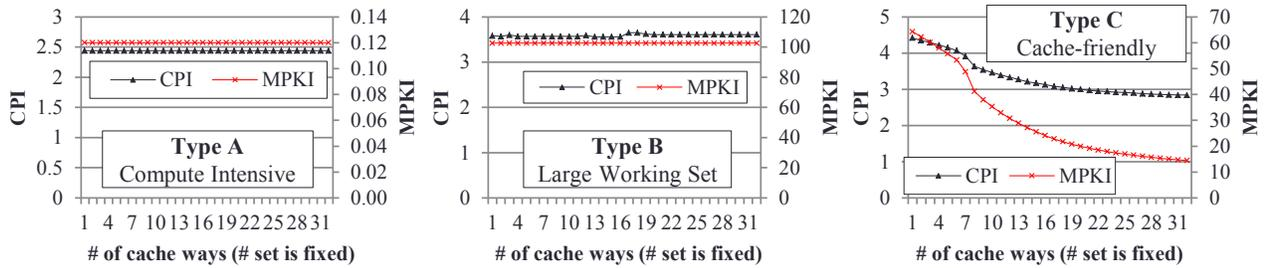
**Figure 2.** Application types based on how the cache affects performance (Ideal CPI is 2 in the baseline. We fix the number of cache sets (4096 sets) and vary the number of cache ways from one (256KB) to 32 (8MB)).
