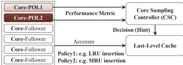
Figure 4. The core sampling framework.
