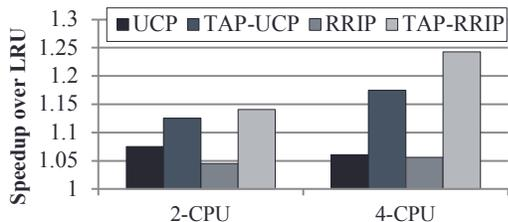
Figure 9. Multiple CPU application results.
