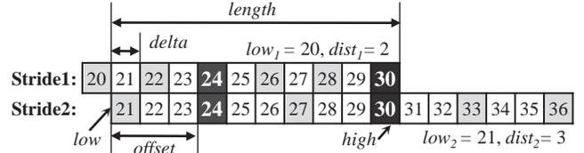
Fig. 6: Two strides in Fig. 5. Lightly shaded boxes indicate accessed locations, and black boxes are conflicting locations. The terms (length, delta, low, high, and offset) are explained in the following paragraphs.
