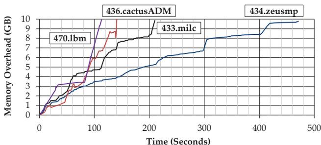
Fig. 19: Memory overhead of the pairwise for 4 SPEC 2006 benchmarks.
