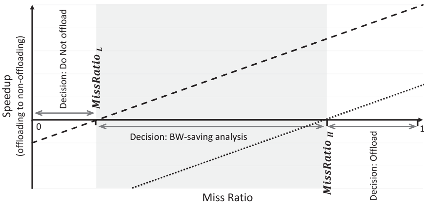
Fig. 5. Speedup of offloading versus non-offloading case and candidate miss ratio for bandwidth-sensitive applications.
